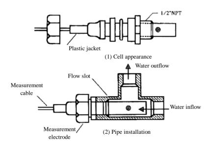
Notes: (1) The electrode should be installed at a lower location in the pipe where the flow speed is steady and air bubbles are seldom generated.
