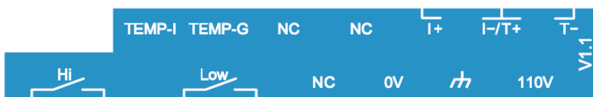
pH/ORP-3510 rear terminal
