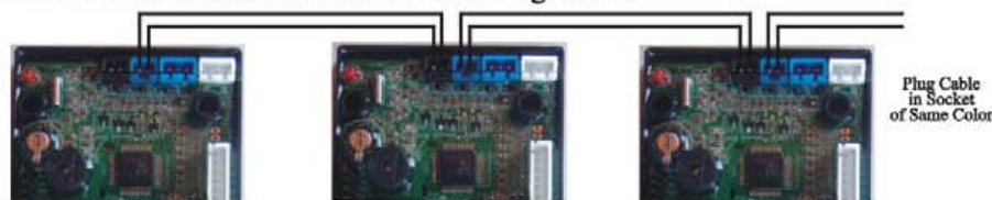
Figure 3-5 Network System Wiring with Interlock Cable
