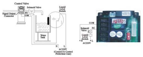
Figure 3-1 Wring of Solenoid Valve on Outlet
